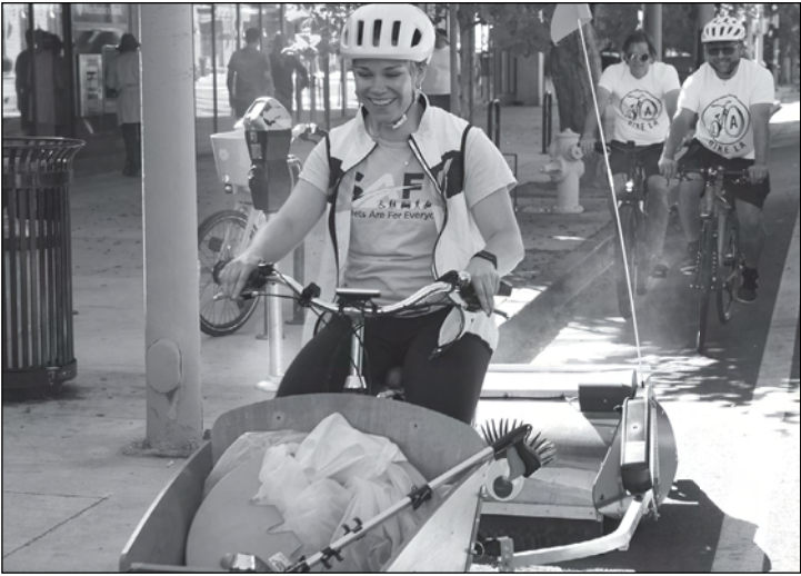
photo courtesy of the 13th Council District office The bike lane street sweeper, towed by Streets Are For Everyone’s Kayla Hankins, fits in spaces inaccessible to traditional sweepers.
